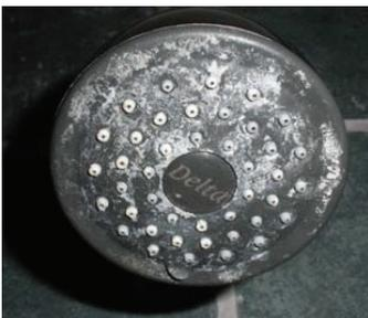
This photo shows the same showerhead on November 7th, 2009, just over five weeks after installation of the Aqua-Rex. The original scale remains on the showerhead but no additional scale has been deposited.
